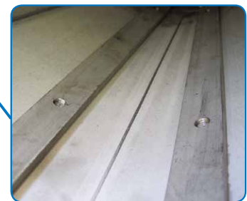
螺栓固定的耐磨条 (内槽视图) Bolted wear bars (internal view of trough)
