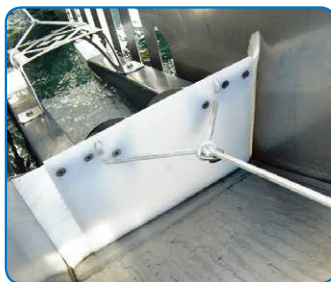
漂浮式刮渣器, 确保各种液 位条件下完全刮除油脂并最 少量的带出水分。 Self-adjusting grease scraper with limited water removal
